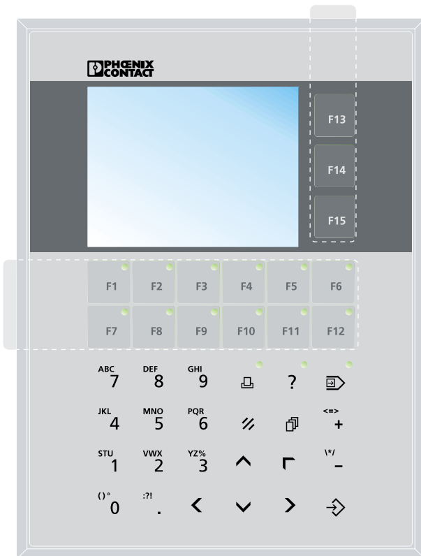
Figure 17 Position of the insert strips in the OT 4M
