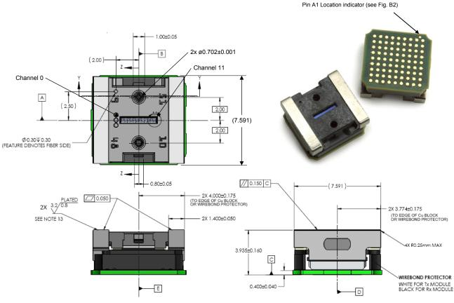
Figure 1. Module Top and Side View
