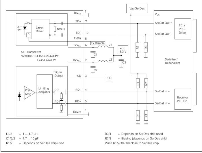
Values of R1/2/3/4 may vary as long as proper 50  $\Omega$  termination to V\_EE or 100  $\Omega$  differential is provided. The power supply filter-
