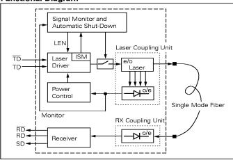
The receiver component converts the optical serial data into PECL compatible electrical data (RD and RDnot). The Signal Detect (SD, active high) shows whether optical data is present<sup>(1)</sup>.
