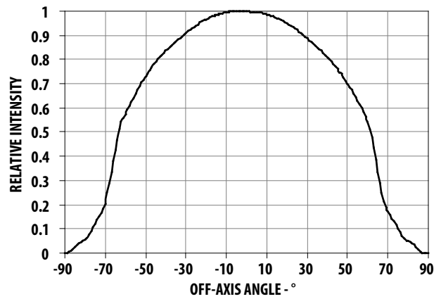
Figure 4. Radiation Pattern for AllnGaP
