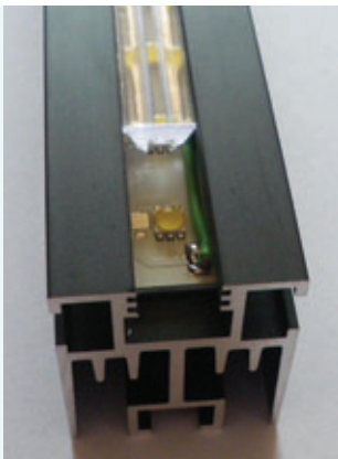
Avago 3W Mini High-Power LEDs in LED Light Strip by Schneider Technologies
