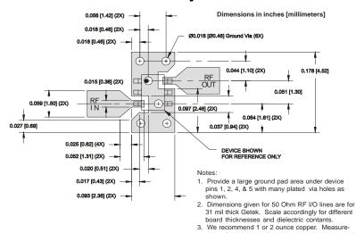
ments for this data sheet were made on a 31 mil thick Getek with 1 ounce copper on both sides.
