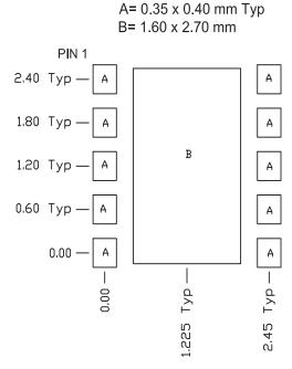
Figure 1. PCB Metal Land Pattern (Top View)
