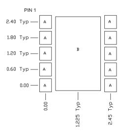
Figure 2. PCB Solder Mask Pattern (Top View)
