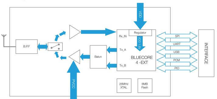
Note: USB and PCM interface are not handled by LM firmware at present
