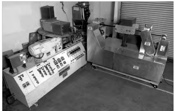
Thermoplastic extruder for microwave absorbing thermoplastic products.
