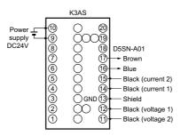
Note: Two inputs are possible on the K3AS, however, due to the output circuit of the D5SN, two current inputs are not possible.
