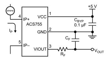
Application 1. The ACS755 outputs an analog signal,  $V_{OUT}$ . that varies linearly with the unidirectional DC primary sampled current,  $I_P$ , within the range specified.  $C_F$  is recommended for noise management, with values that depend on the application.
