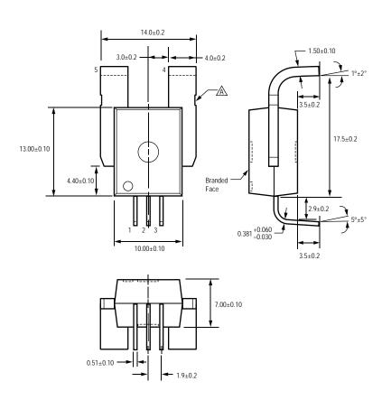
Creepage distance, current terminals to signal pins: 7.25 mm Clearance distance, current terminals to signal pins: 7.25 mm Package mass: 4.63 g typical
