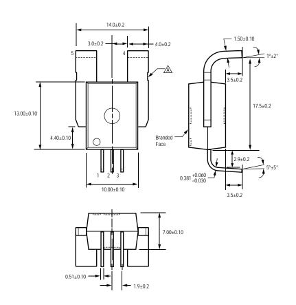
Creepage distance, current terminals to signal pins: 7.25 mm Clearance distance, current terminals to signal pins: 7.25 mm Package mass: 4.63 g typical
