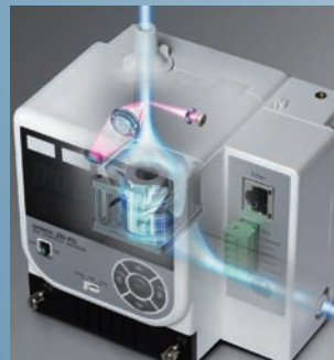
Intake air is irradiated with laser light and the level of scattered light from particles is measured.
