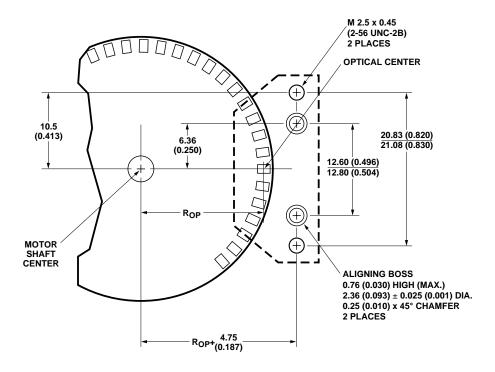
Figure 2. Mounting plane side B.
