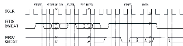
Figure 21. Read Data Waveform with Extended Index
