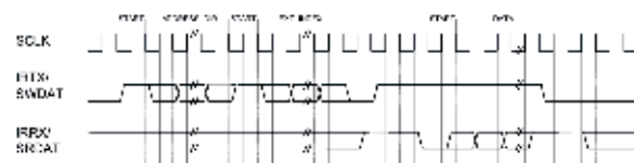
Figure 21. Read Data Waveform with Extended Index
