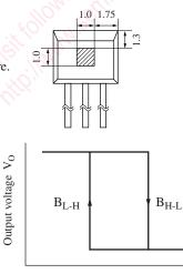
Applying direction of magnetic flux
