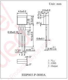
Note) The package of this product will be changed to lead-free type (SSIP003-P-0000H). See the new package dimensions section later of this datasheet.
