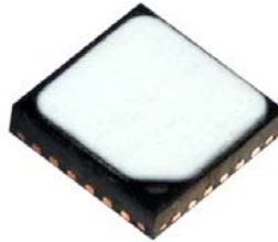
Figure 7. Si7015 with Factory-Installed Protective Cover
