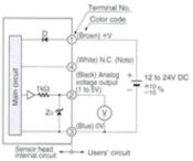
Note: In case the pressure sensor head is used independently, insulate the white wire (Terminal No.4) and keep it open.
