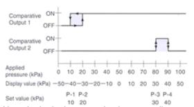
Note: In the leak test mode, the zero-adjustment function is applied only to Comparative Output 2. Comparative Output 1 operates with the atmospheric pressure as the reference.
