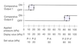
Note: In the hysteresis mode, Set Value P-3 and Set Value P-4 are shifted. The output is set to the window comparator mode or the leak test mode.
