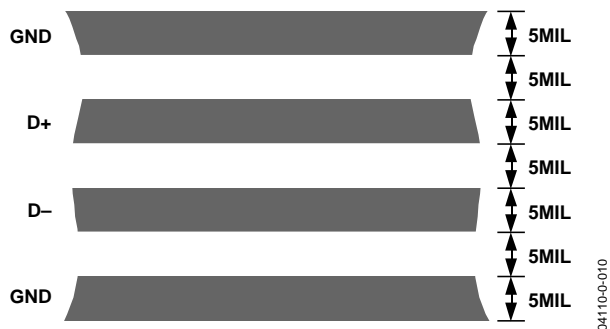
Figure 24. Typical Arrangement of Signal Tracks
