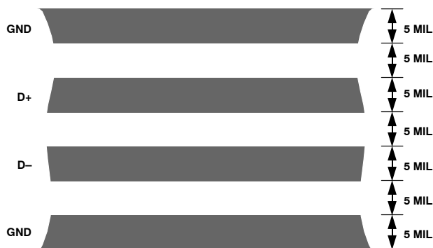
Figure 22. Typical Arrangement of Signal Tracks
