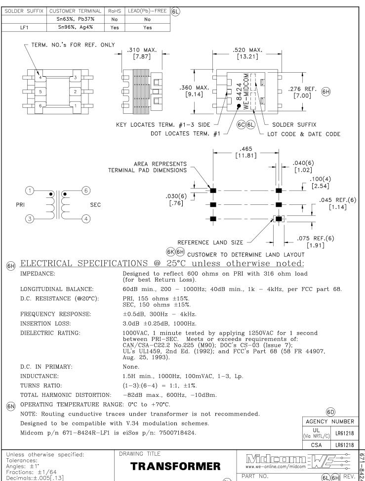
This drawing is dual dimensioned. Dimensions in brackets are in millimeters.
