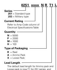
The default lead length for Ammo pack and Loose pack is now T1 for 251 series, and remains T3 for 253 series, therefore: T1 = 52.4mm (2.062"), 251 series only\* Blank = 52.4mm (2.062") for 251 series\* or 73mm (2.874") for 253 series\*\*
