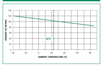
1. Rerating depicted in this curve is in addition to the standard derating of 25% for continuous operation.
