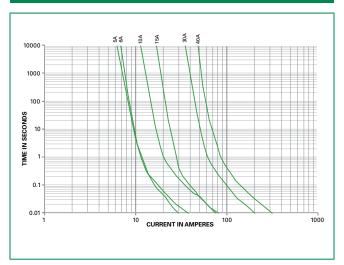
Note: Rerating depicted in this curve is in addition to the standard derating of 25% for continuous operation.
