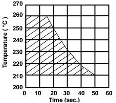
(4) Standard Temperature Profile for Soldering
