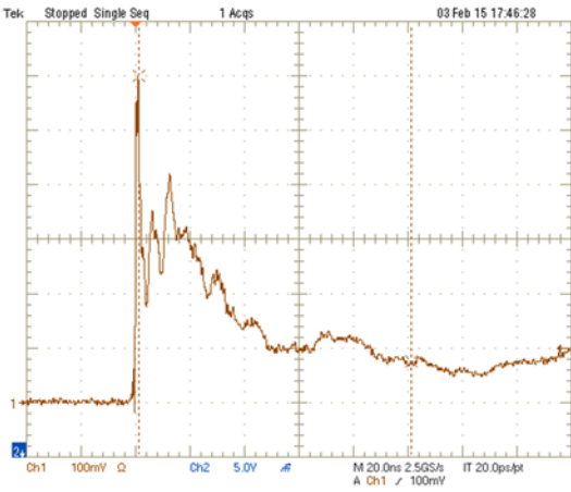
Figure 1. IEC61000-4-2 +8kV Contact ESD Clamping Voltage
