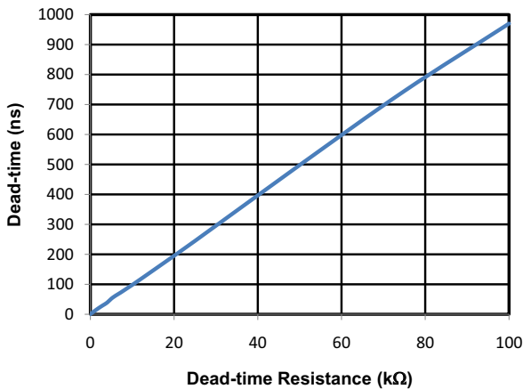
Figure 37. Dead Time vs. Resistance ( R_{DT} )
