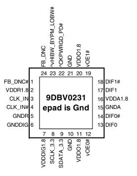
24-pin VFQFPN, 4x4 mm, 0.5mm pitch ^ prefix indicates internal 120KOhm pull up resistor ^v prefix indicates internal 120KOhm pull up AND pull down resistor (biased to VDD/2) v prefix indicates internal 120KOhm pull down resistor
