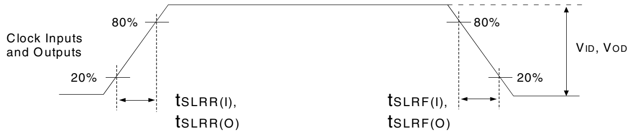
Figure 8. Input and Output Slew Rates
