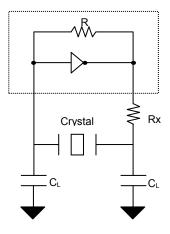
$$\begin{split} C_\text{L} &= 2^*(C_P - C_S), \\ \text{Where } C_P &= \text{Load capacitance of crystal} \\ C_S &= \text{Stray capacitance due to } C_\text{IN,} \text{ PCB, Trace etc.} \end{split}$$
