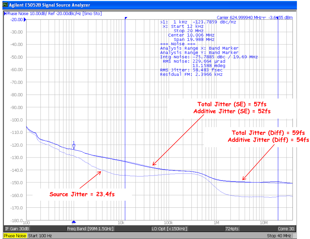
Figure 15. Source, Additive, and Total Jitter (625 MHz)
