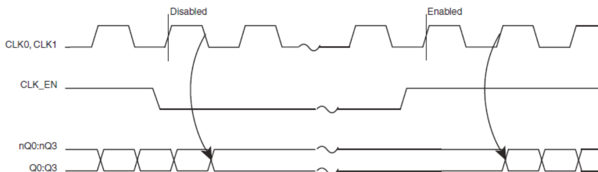
FIGURE 1. CLK_EN TIMING DIAGRAM
