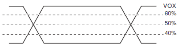
OUTPUT CROSSOVER VOLTAGE
