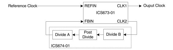
Note that in both examples, Divide B is connected to the output of the ICS673. This is because Divide B has a higher operating frequency than Divide A.
