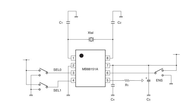
$C_1,\,C_2$  : Oscillation stabilization capacitance (refer to "Oscillation Circuit".)
