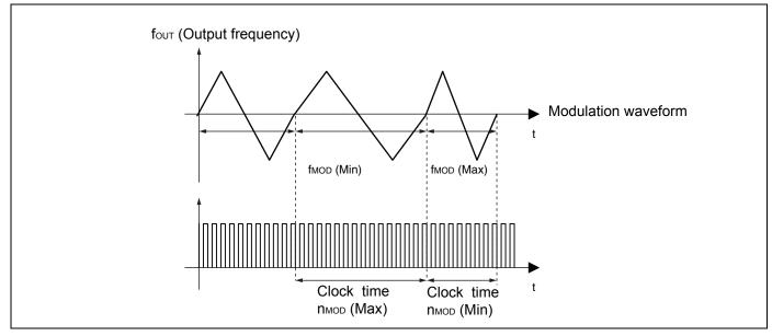
MB88151A contains the modulation period to realize the efficient EMI reduction.
