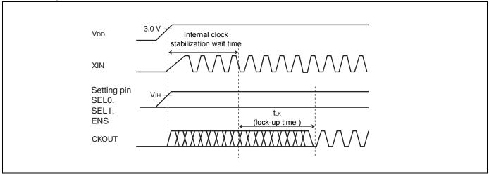
If the setting pin is fixed at the "H" or "L" level, the maximum time after the power is turned on until the set clock signal is output from CKOUT pin is (the stabilization wait time of input clock to XIN pin) + (the lock-up time "tlk"). For the input clock stabilization time, check the characteristics of the resonator or oscillator used.
