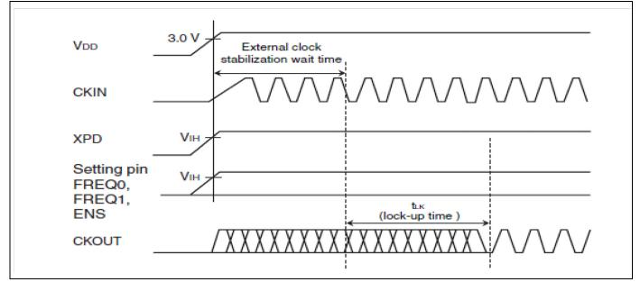
If the XPD pin is fixed at the "H" level, the maximum time after the power is turned on until the set clock signal is output from CKOUT pin is (the stabilization wait time of input clock to CKIN pin) + (the lock-up time " $t_{LK}$ "). For the input clock stabilization time, check the characteristics of the resonator or oscillator used.
