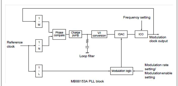
A glitchless IDAC (current output D/A converter) provides precise modulation, thereby dramatically reducing EMI.
