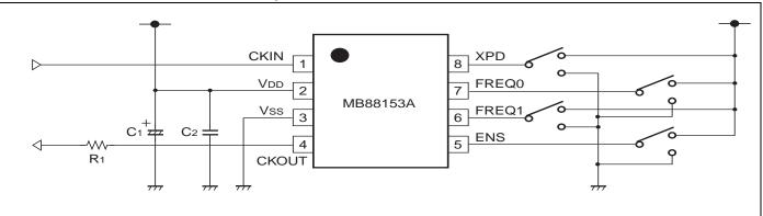
$C_1$ : Capacitor of 10  $\mu F$  or higher
