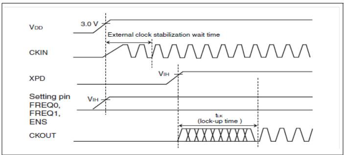
When XPD pin controls the power-down, stable clock is output from CKOUT pin after becoming XPD pin = "H" level (in the maximum after lock-Up time ( $t_{LK}$ )).
