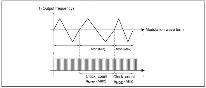
MB88153A contains the modulation period to realize the efficient EMI reduction.
