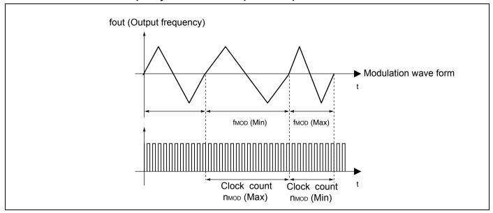
MB88154A contains the modulation period to realize the efficient EMI reduction. The modulation period  $f_{\text{MOD}}$  depends on the input frequency and changes between  $f_{\text{MOD}}$  (Min) and  $f_{\text{MOD}}$  (Max) . Furthermore, the average value of  $f_{\text{MOD}}$  equals the typical value of the electrical characteristics.
