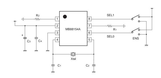
C<sub>1</sub>, C<sub>2</sub> : Oscillation stabilization capacitance (refer to "Oscillation Circuit".)
