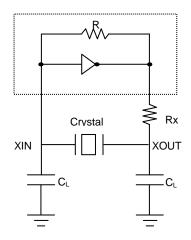
$$\begin{split} C_L &= 2^*(C_P - C_S), \\ \text{Where } C_P &= \text{Load capacitance of crystal from crystal vendor datasheet.} \\ C_S &= \text{Stray capacitance due to } C_{\text{IN}}, \text{PCB}, \text{Trace, etc.} \end{split}$$
