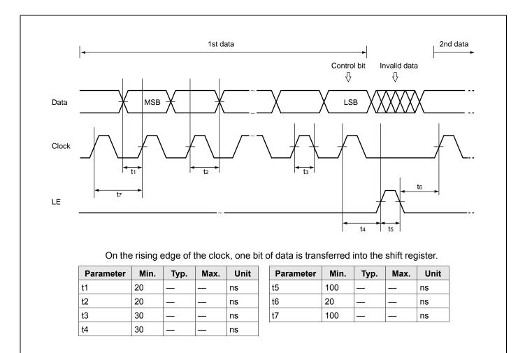
Note: LE should be "L" when the data is transferred into the shift register.
