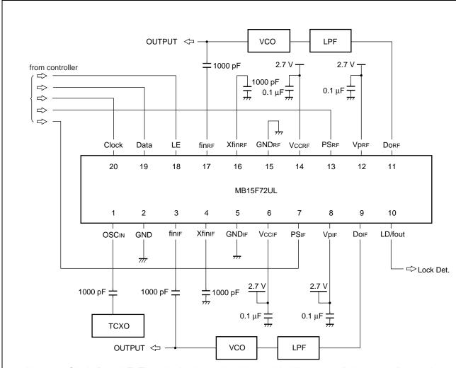
Notes: • Clock, Data, LE: The schmitt trigger circuit is provided (insert a pull-down or pull-up register to prevent oscillation when open-circuit in the input) .
