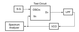
$\begin{array}{lll} \text{fvco} = 720.5 \text{ MHz} & \text{Vcc} = 3.0 \text{ V} \\ \text{Kv} = 31 & \text{Vvco} = 3.0 \text{ V} \\ \text{fr} = 12.5 \text{ kHz} & \text{Ta} = +25 \text{ °C} \\ \text{fosc} = 19.2 \text{ MHz} & \text{CP} : 6 \text{ mA mode} \\ \text{LPF} \end{array}$
