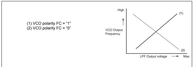
Note: Give attention to the polarity for using active type LPF.
