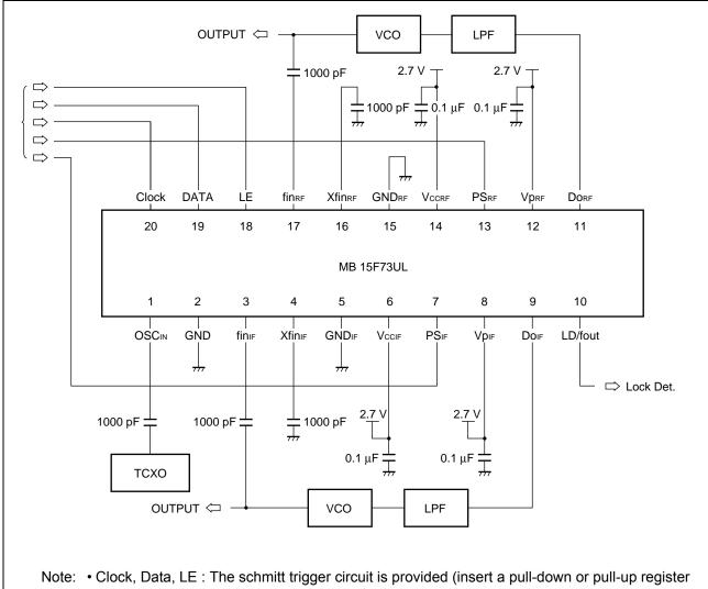
to prevent oscillation when open-circuit in the input).
