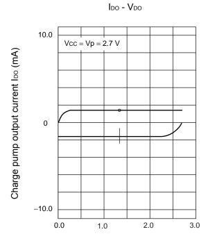
Charge pump output voltage V<sub>DO</sub> (V)
