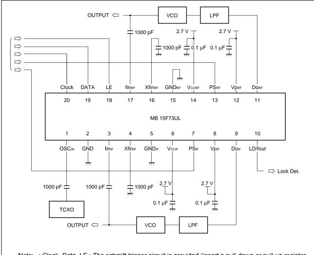
Note: • Clock, Data, LE: The schmitt trigger circuit is provided (insert a pull-down or pull-up register to prevent oscillation when open-circuit in the input).
