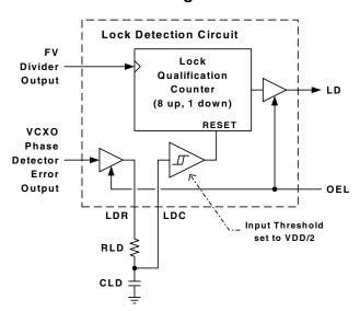
If the lock detection circuit is not used, the LDR output may remain unconnected, however the LDC input should be tied high or low. If the PCB was designed to accommodate the RLD and CLD components but the LD output will not be used, RLD can remain unstuffed and CLD can be replaced with a resistor (< 10 kohm).
