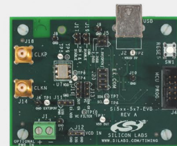
Si570 I²C OSCILLATOR EVALUATION BOARD
