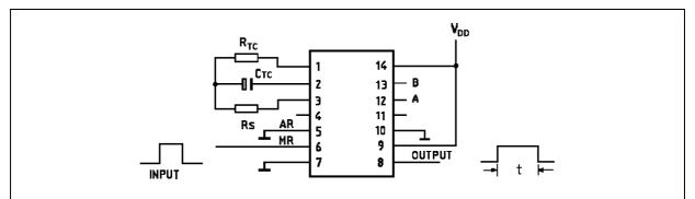
A positive MASTER RESET pulse clears the counter and latch. The Output goes high and keeps up till the number of pulses, selected by A and B, are counted. This circuit is retriggerable and is as accurate as the input frequency. If a
