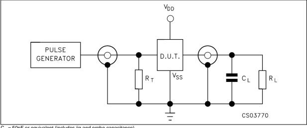
$\begin{array}{l} C_L = 50 pF \mbox{ or equivalent (includes jig and probe capacitance)} \\ R_L = 200 K\Omega \\ R_T = Z_{OUT} \mbox{ of pulse generator (typically 50 \Omega)} \end{array}$
