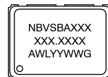
6 PIN CLCC LN SUFFIX CASE 848AB
