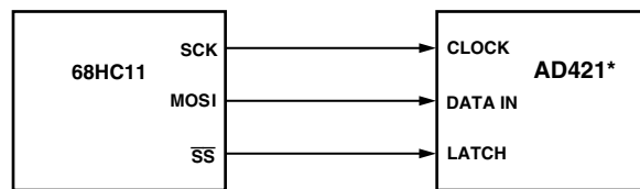
Figure 8. AD421 to 68HC11 Interface
